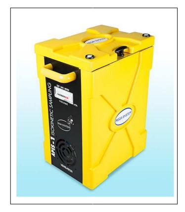
The installation of an optional electronic card for the acquisition of signals of 4-20mA / 1-10V allowing the instrument to acquire and save in the sampling report the data coming from analyser of other manufacturer and to use some of the parameters acquired for the calculation of the isokinetic flow in real time.
